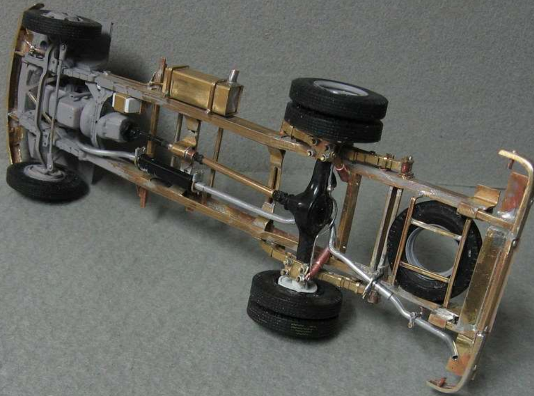
Soldered brass chassis, bumpers, etc.
